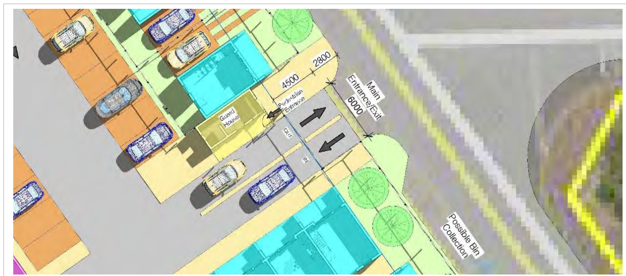
Figure 3.11: Main Vehicular Entrance and Exit Gate (Source: JSA Associates)
