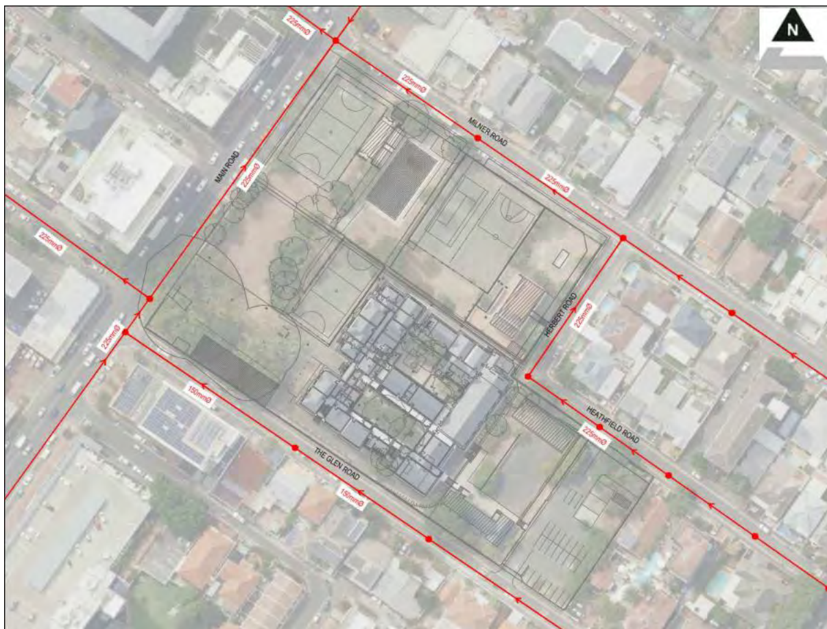
Figure 74: Existing Sewer Infrastructure
