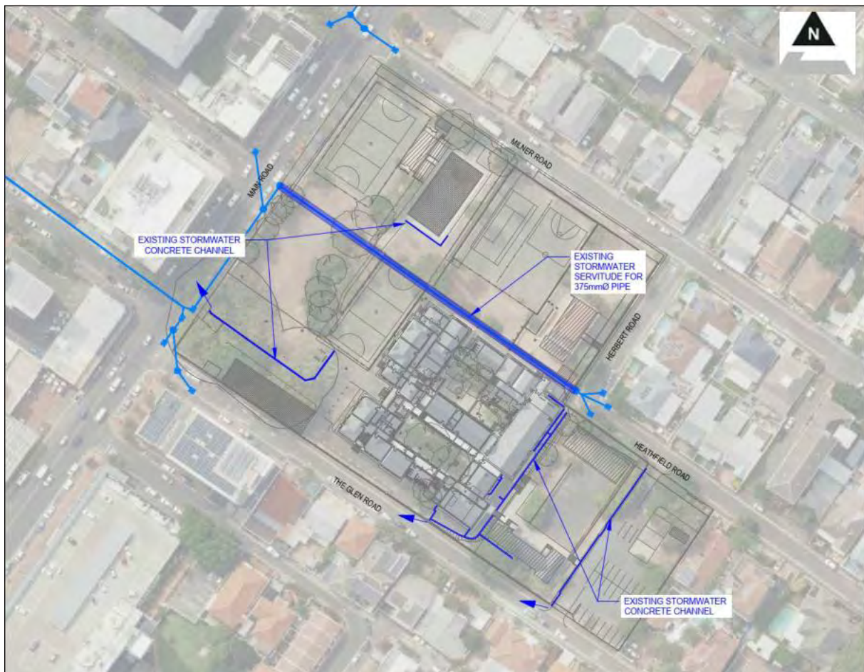
Figure 75: Existing Stormwater Infrastructure
