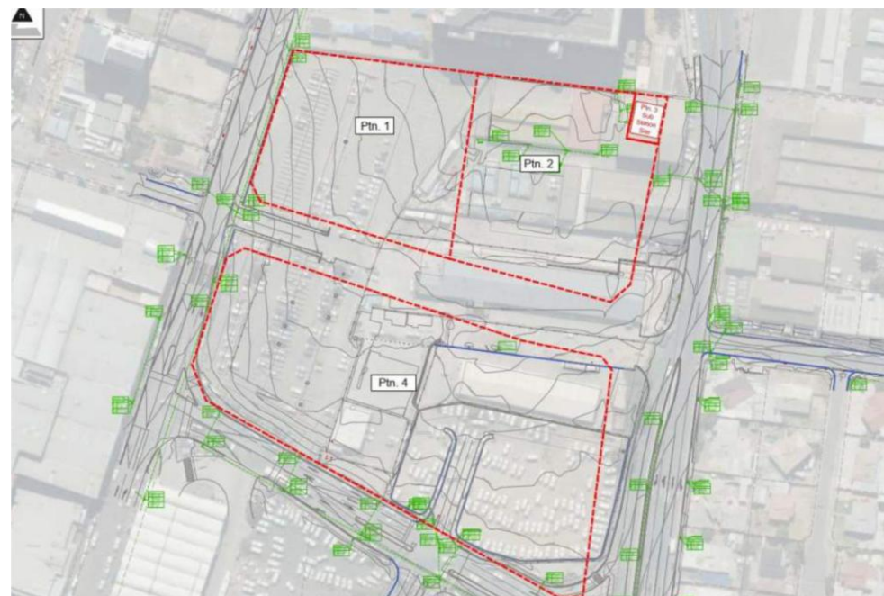
Figure 3.23: Existing stormwater layout (Zutari, 2026)
