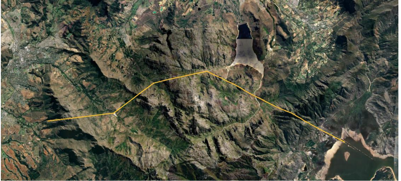
Figure 3 Extent of the RSE Tunnel System
